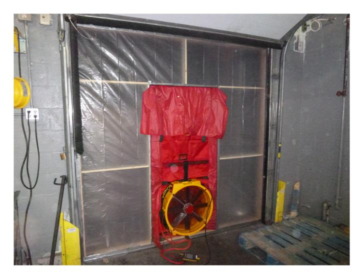
Blower Door mounted in custom frame that fits dock opening with sealed test assembly
