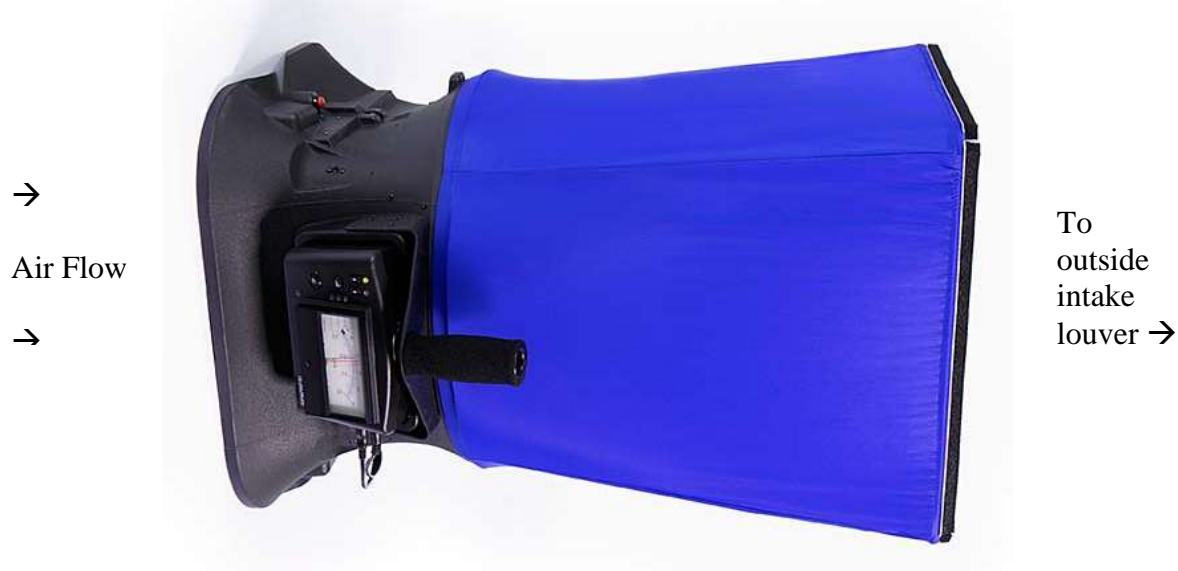
Figure 5. Flow hood traverse orientation. 4
