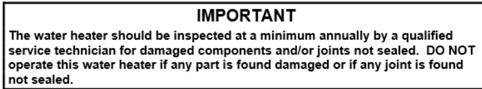
Figure 1: Storage Water Heater Maintenance Recommendation
