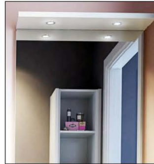
External Mirror Lights - D 40 W Max Allowed (2 X 20 W)
