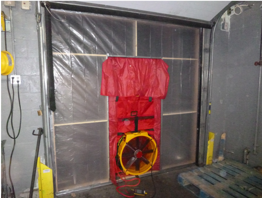
Figure 2: Dock door air leakage test apparatus
