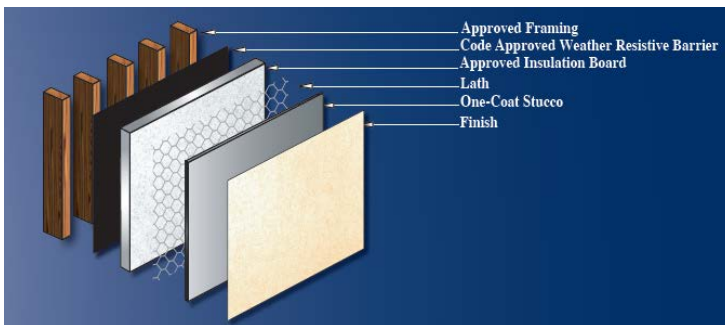
Figure 2: Typical one-coat stucco assembly detail.
