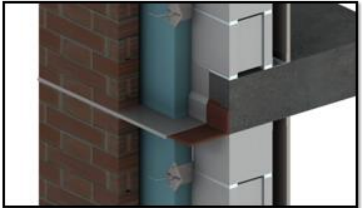
Thermal Bridging due to a shelf angle that supports brick veneer
