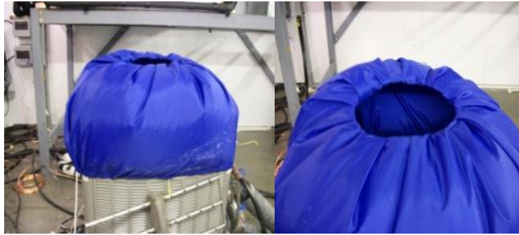
Figure 2. An Example of a Condenser Air Exit Restrictor
