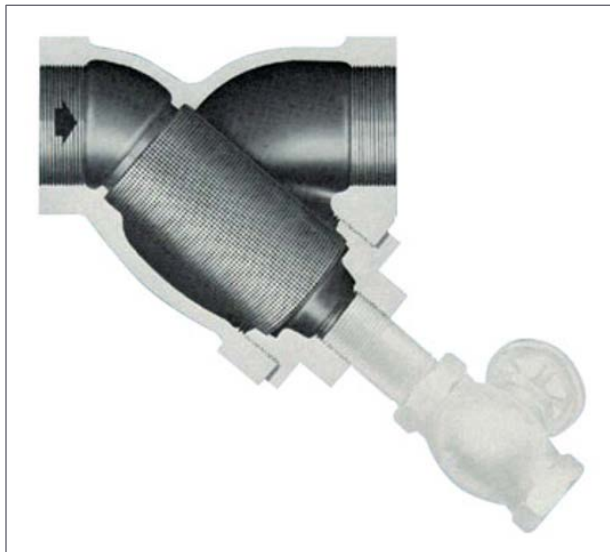
Figure 3: Strainer with blow-off valve to the bottom.
