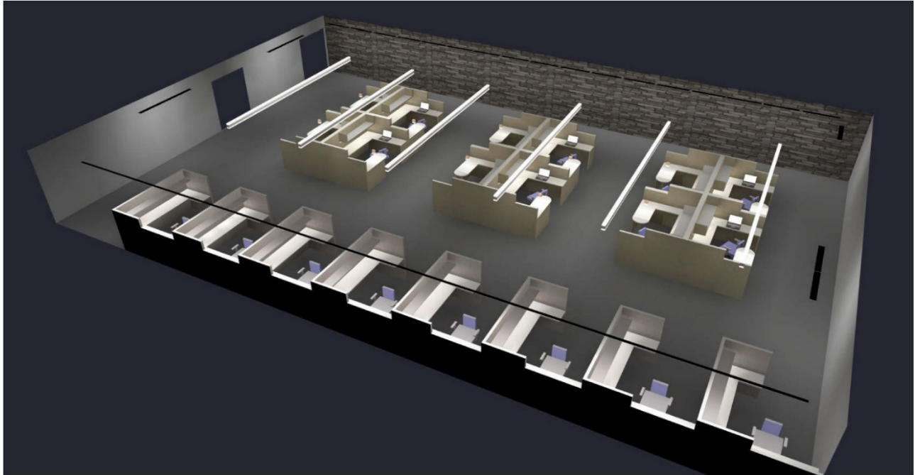
Figure 47: Perspective View 2022 Design A1 Pendant + Undercabinet Lighting with Brick Wall.
