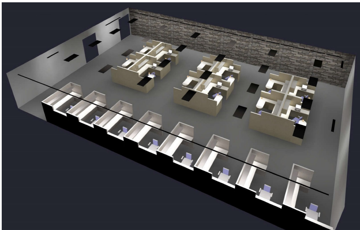
Figure 51: Perspective View 2022 Design B1 Troffer + Undercabinet Lighting with Brick Wall.
