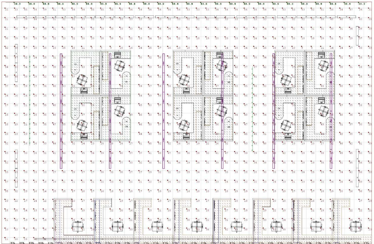
Figure 46: Plan View 2022 Design A1 (Pendant + Task Lighting).
