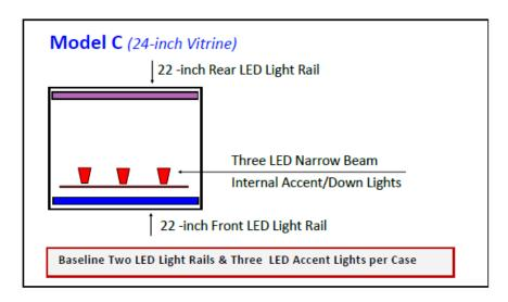
Figure 36: Model C (24" vitrine) used for updating very valuable display lighting power densities.
