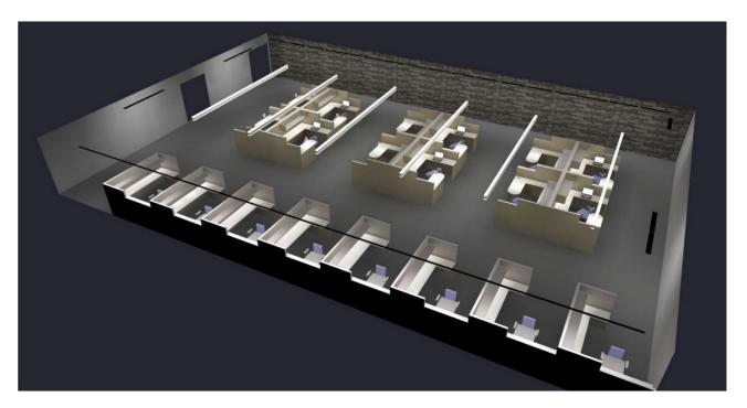
Figure 47: Perspective View 2022 Design A1 Pendant + Undercabinet Lighting with Brick Wall.
