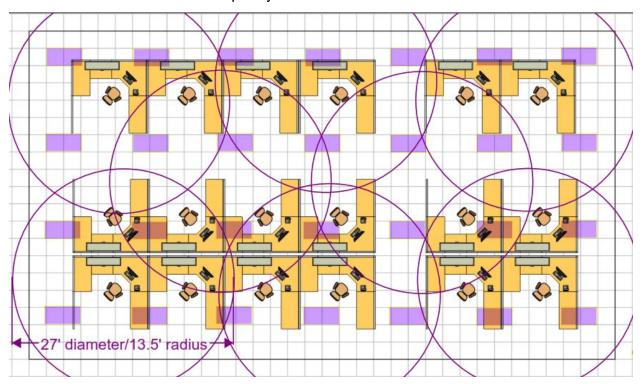
Figure 17: Floor plan of Model Office A with a sample occupancy sensor layout.
