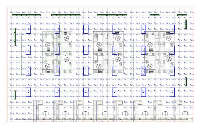
Figure 44: Plan View 2019 Design B (Recessed LED Basket Troffers Task Ambient Lighting)
