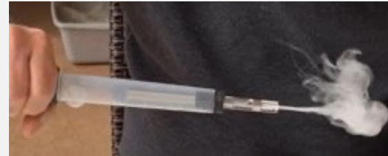
Example of a fog puffer for finding leaks (Source: The Energy Conservatory, https://store.energyconservatory.com/tec-fog-puffer.html .)
