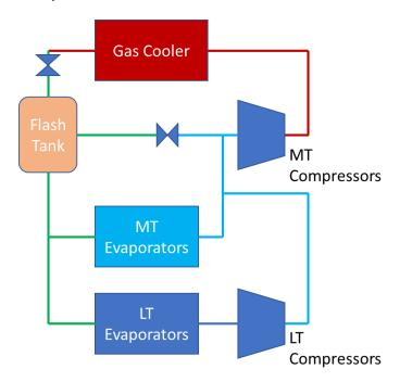
Figure 1: Transcritical CO<sub>2</sub> booster refrigeration system diagram.
