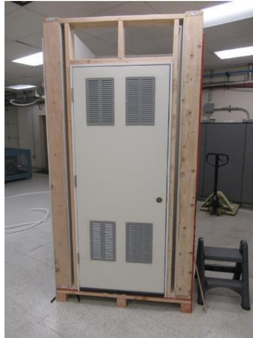
Figure 43: Ventilation grilles on the door of the closet used in laboratory tests.
