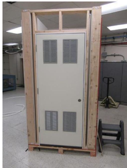
Figure 46: Ventilation grilles on the door of the closet used in laboratory tests.
