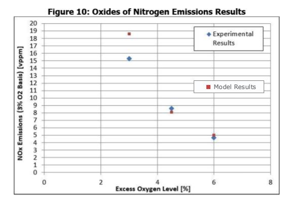
Image from CEC Project Report: <u>Demonstration of a Novel Ultra-Low Oxides of Nitrogen Boiler for Commercial Buildings, 2021</u>
