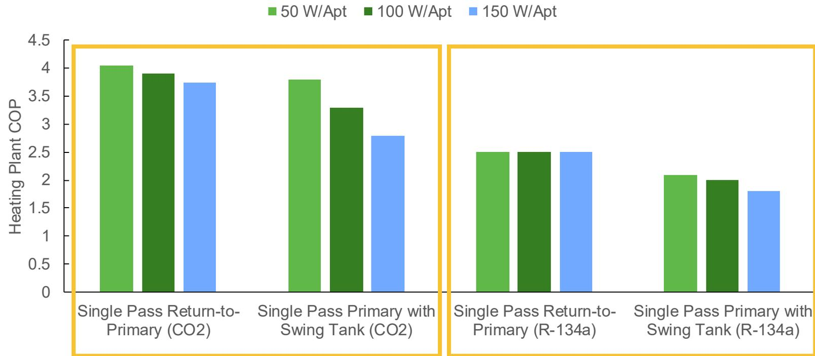
Lab test results on Heating Plant COP for various central HPWH configurations with different refrigerants
